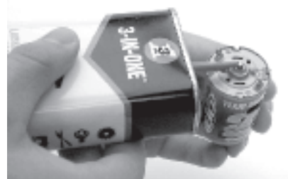
Apply a small amount of lightweight oil to each bushing for lubrication.
