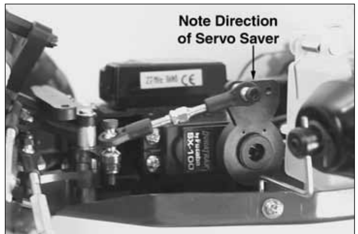
7. Place the servo saver onto the steering servo as shown.
