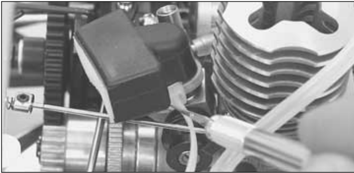
❑ 5. Remove the air filter and tie strap from the parts bag. Thoroughly soak the air filter foam with some oil (not included) and then squeeze out the excess oil. A light machine oil (like 3-IN-ONE) will work well. Special oils made for air filters are also available in most hobby and motorcycle shops. Place the air filter onto the carburetor and secure it in place with the tie strap. Cut off the excess part of the strap.
