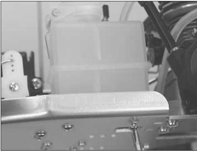
❑ 4. Re-install the fuel tank.
