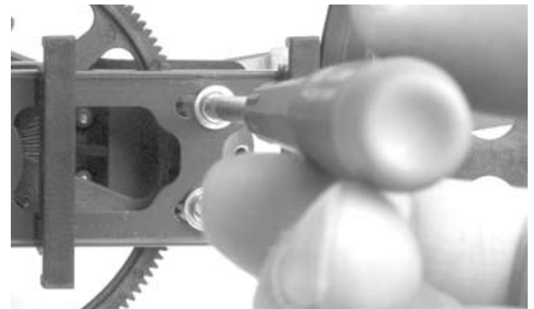
Using a Phillips head screwdriver fully tighten the motor bolts in place where the gear mesh is best.
