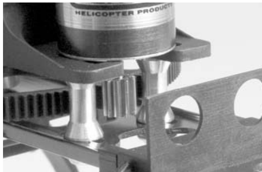
Using the two included silver aluminum motor standoffs (pictured), align the motor for best possible gear mesh.
